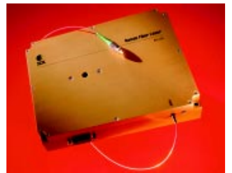
Figure 2: Shown above is a high power (1.5 W) fiber laser operating at 1455 nm. This allows amplification of 1550 nm optical signals through 20 km of standard single mode optical transmission fiber via stimulated Raman scattering (SRS). SRS amplification is expected to allow 40 Gb/sec transmission over many wavelength channels to further enhance the transmission capacity per fiber.
