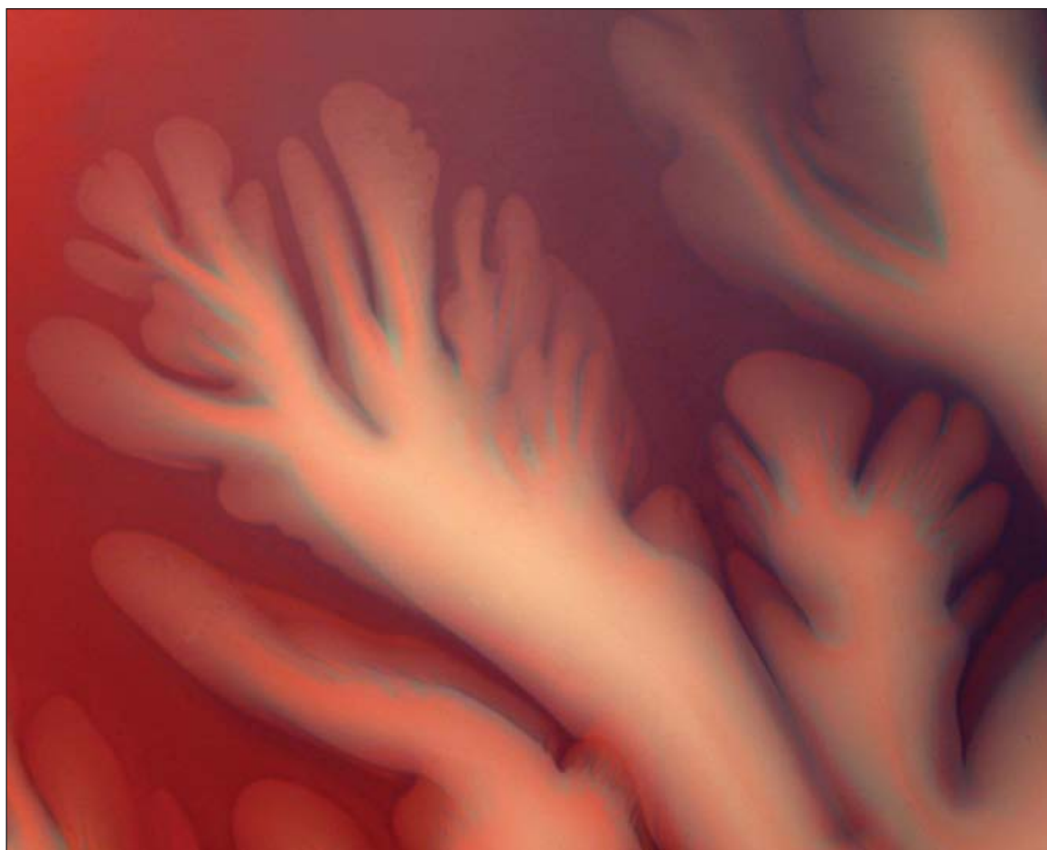
Saffman-Taylor instability in a Hele-Shaw cell. This image was a winner in the 2004 Gallery of Fluid Motion.
