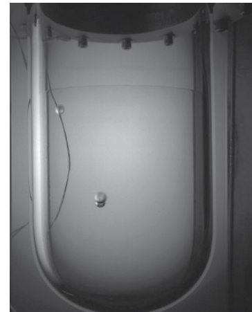
A bubble chamber dark matter detector at the Chicagoland Observatory for Underground Particle Physics experiment at the University of Chicago
