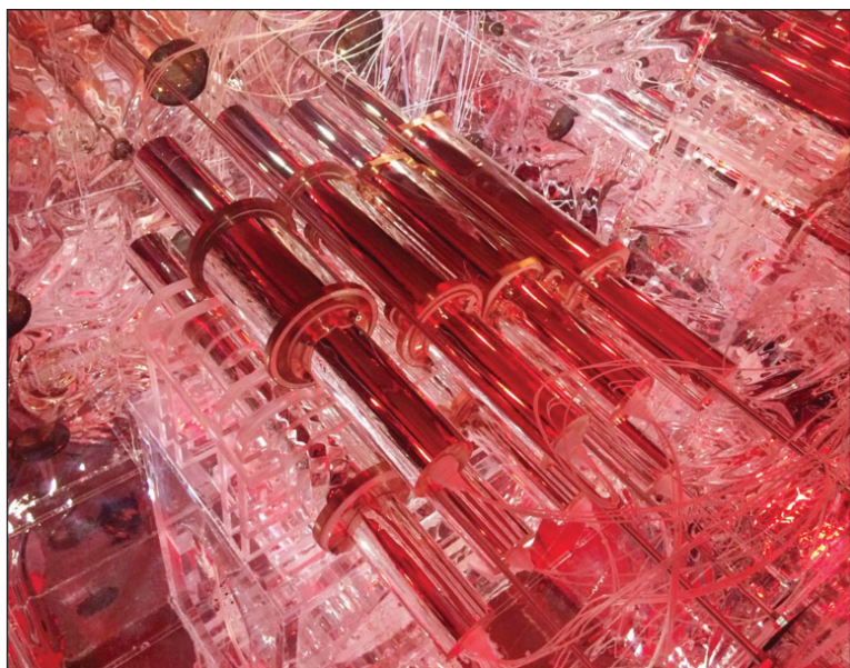
Two experiments, COSINE-100 (pictured) and ANAIS, employ the same detector material in an effort to replicate the DAMA/LIBRA signals claimed to result from dark matter. IMAGE: COSINE-100
